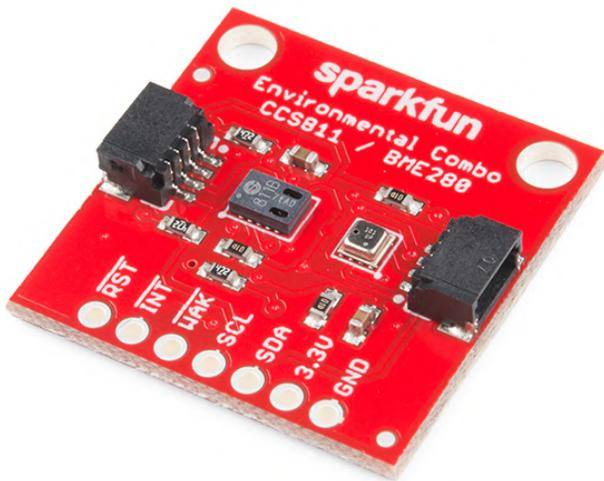
**Figure 2 - The SFE Environmental Combo Breakout. Image courtesy of SparkFun Electronics.**
