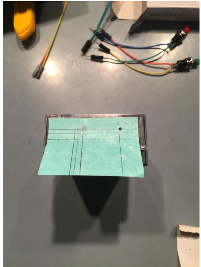
**Figure 2 - Use a sticky note to position the buttons in your case**
