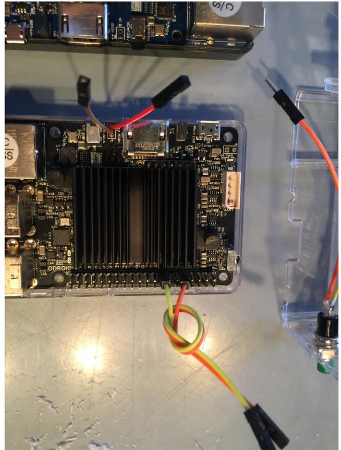
Figure 7 - Place one jumper on pin 9, GROUND, of the 40-pin GPIO header
