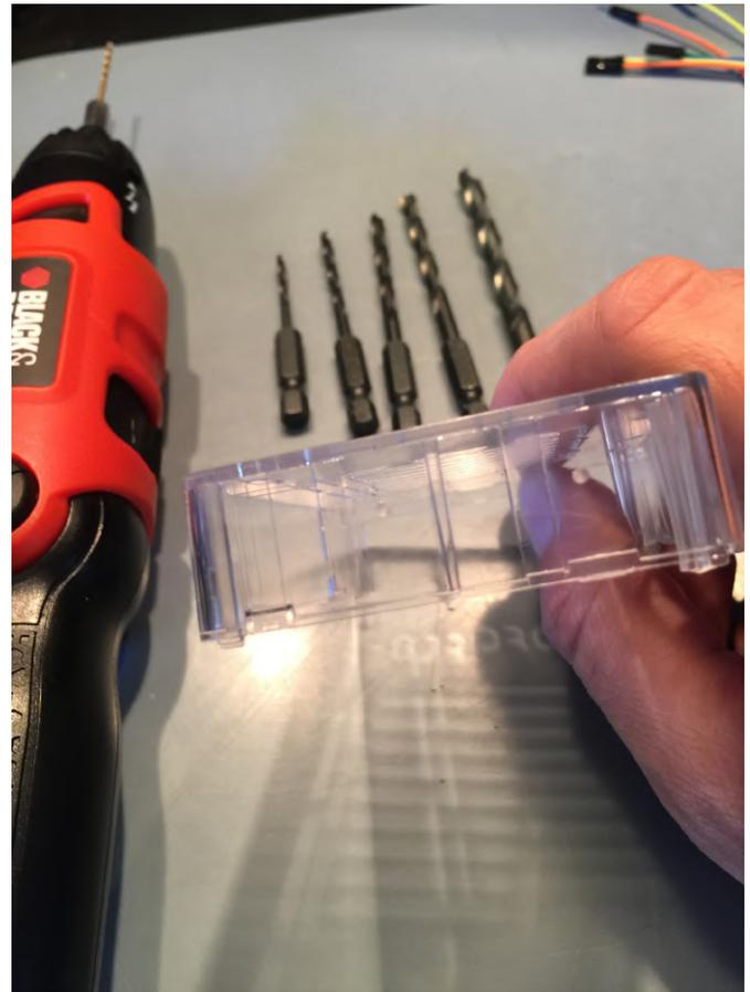
**Figure 4 - Drill through the paper into the plastic, just deep enough to leave a bit of a visible mark**
