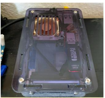
Figure 3 - XU4 cloudshell with Noctua cooler
