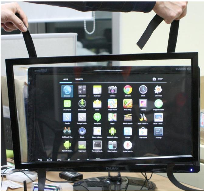
Figure 14 - 23-inch touch screen panel with velcro belts
