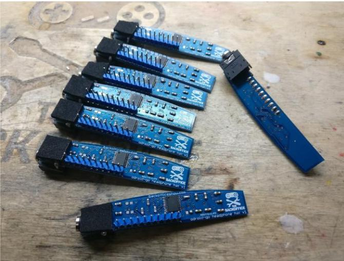
**Figure 8 - Built Odroid Audio Hats - Closeup of the hand assembled v1 boards**
