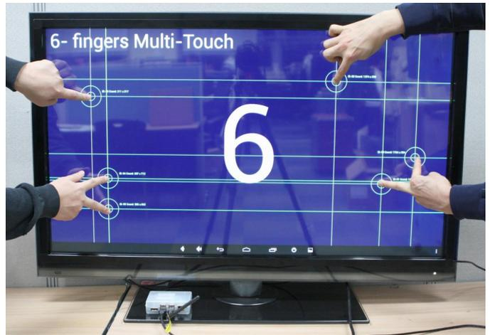
Figure 13 - Testing the touch screen
