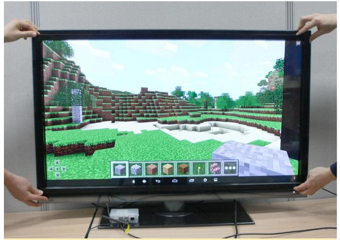
Figure 12 - Aligning the touch screen with the monitor
