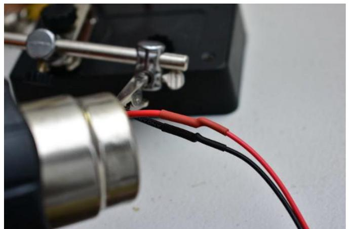
**Figure 5 - The JST plug goes to the voltage converter inside the aluminum box. All cable bonds are protected with heat-shrink tubing**
