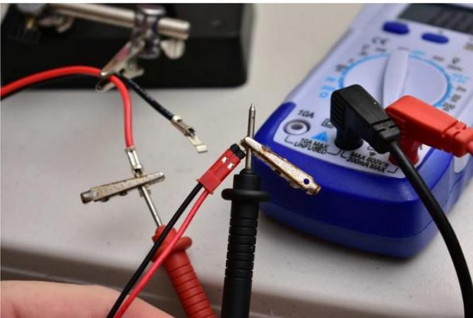
Figure 8 - Here I am testing for continuity
