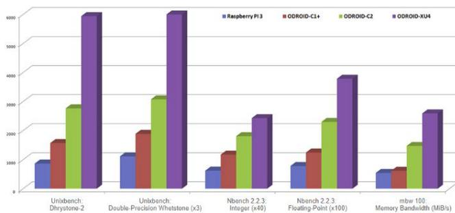
**Figure 1 - Performance of ODROID-HC2 is identical to XU4 (which is more of a media pc)**
