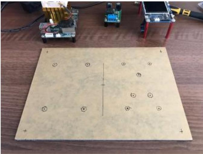
**Figure 6 - The acrylic sheet ready for drilling**
