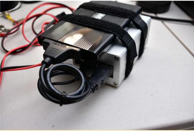
Figure 18 - The ODROID-C2 supports eMMC storage and this one has a 16 GB card which is used for system files. For storage, an external SSD SATA hard drive is used with a SATA to USB adapter
