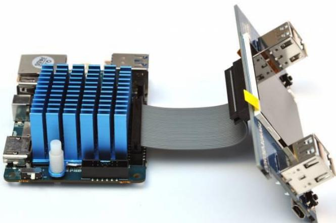
Figure 2 - Use a 30-pin flat cable (E) to connect the XU4 and the LCD board (C). Then remove the LCD surface protect film. The ODRROID-XU4 is sold separately
