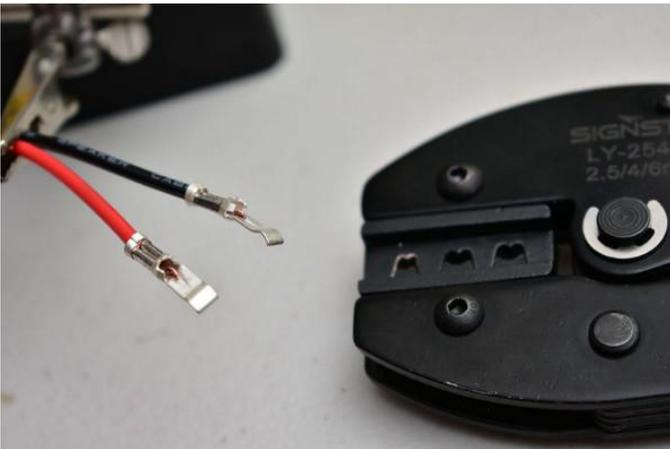
Figure 7 - I crimped then and added a bit of solder for best conductivity
