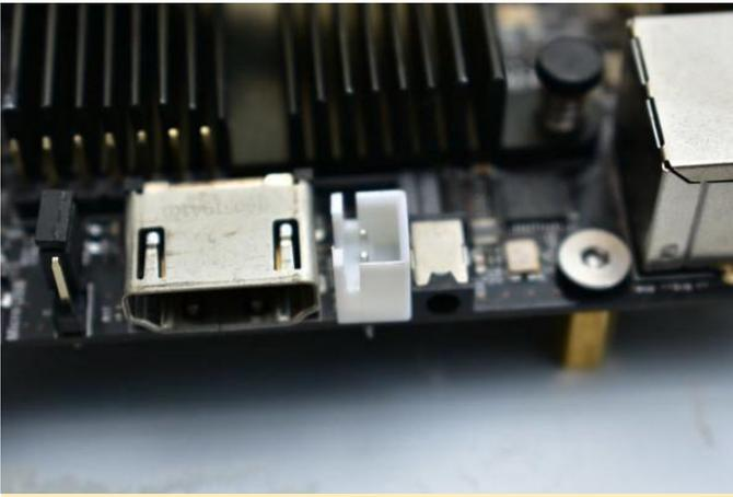
Figure 12 - The serial console and power plugs were replaced as shown
