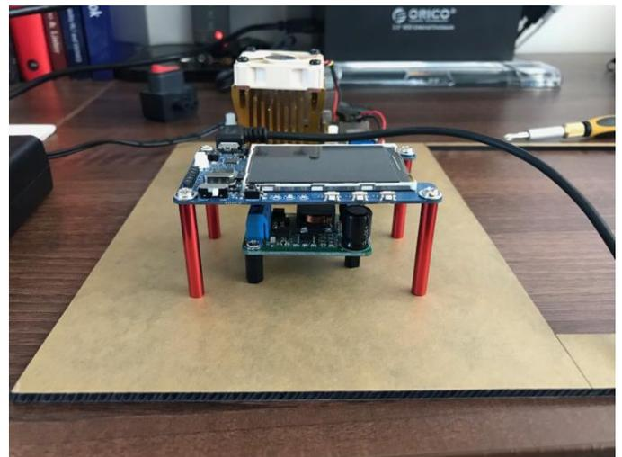
**Figure 5 - Another view of the standoffs for the XU4 and the DC-DC converter**
