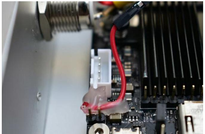
Figure 11 - The serial console and power plugs were replaced as shown
