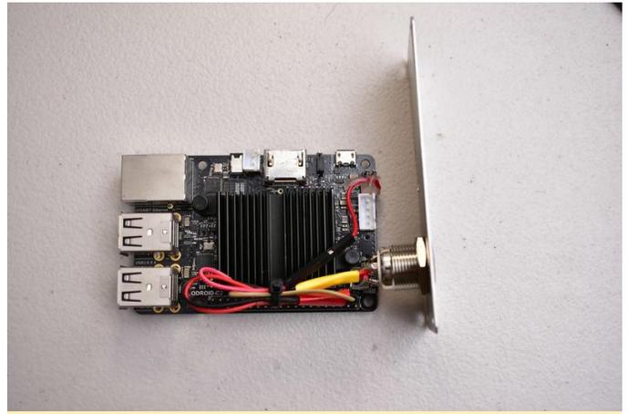
**Figure 3 - This is the ODROID C2 with power indicator and button installed. The switch is not connected to anything and left for future use (maybe via GPIO). The power indicator is soldered to heartbeat LED on the board**
