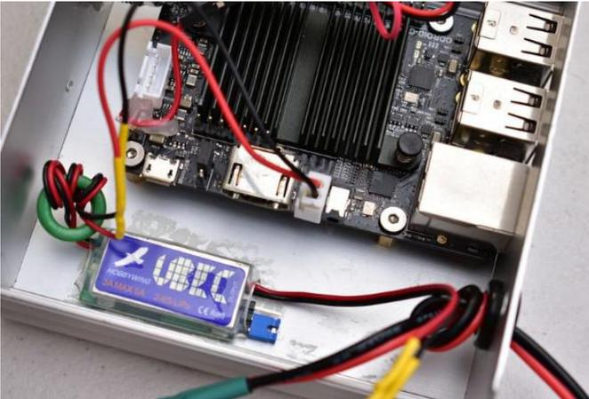
Figure 13 - Here is the Voltage converter mounted with double-sided tape. The converter takes the 12 volts from the solar system and reduces it to 5 volts
