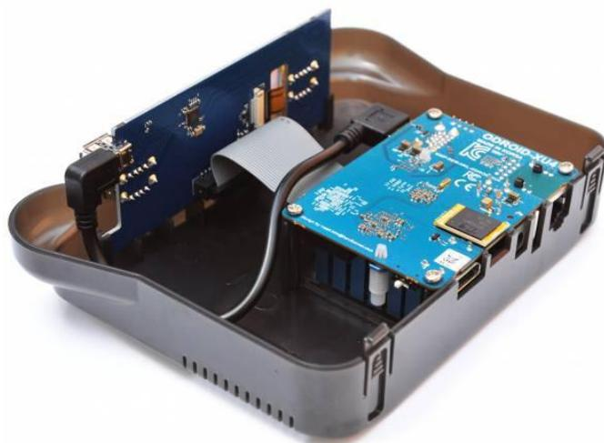
Figure 5 - Connect the XU4 board and the LCD board with the USB2.0 cable (D)
