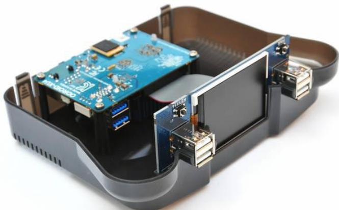
Figure 4 - Connect the XU4 board and the LCD board with the USB2.0 cable (D)
