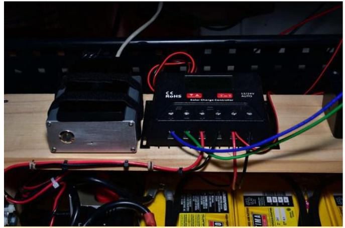
Figure 20 - Here is the microserver placed next to the solar system charge controller and connected to the Anderson power distribution box
