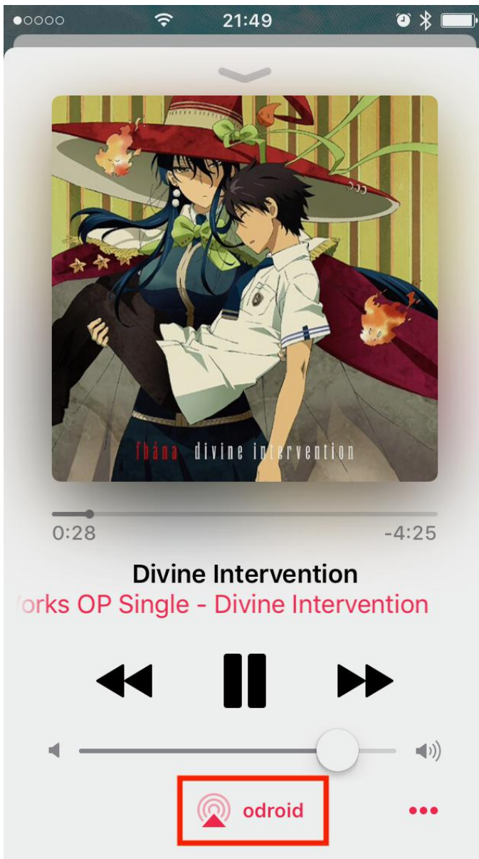
Figure 5 – Sending audio playback via Bluetooth from iTunes to the ODROID-XU4
