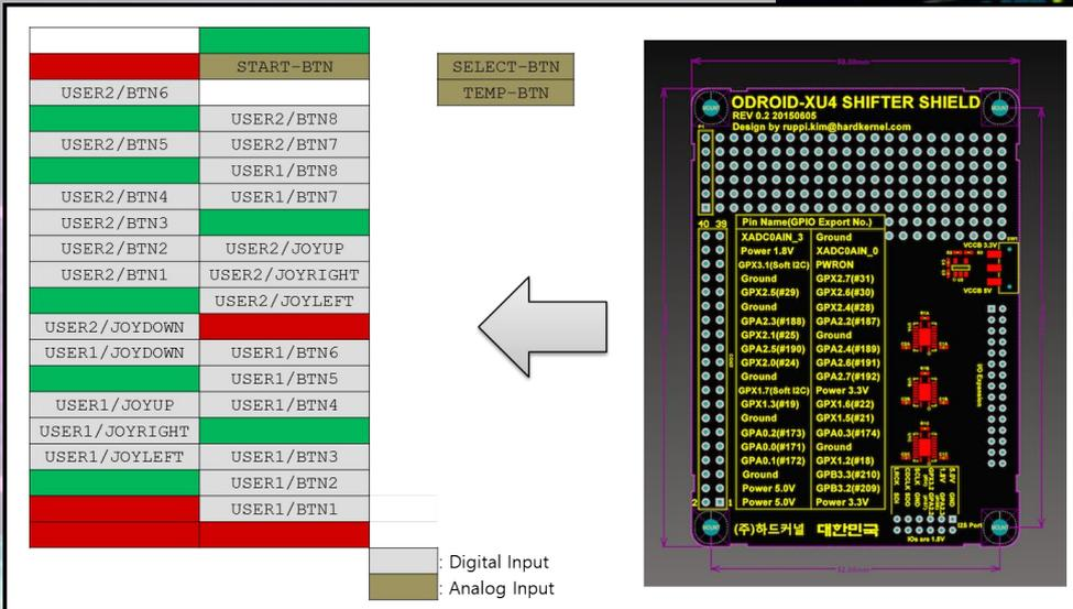
**External GPIO mappings for the Buttons and Joysticks**
