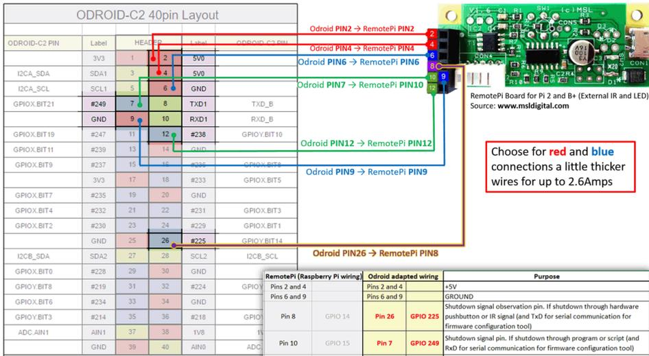
Figure 2 - GPIO rewiring
