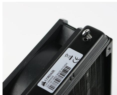
**Figure 3 - The self-tapping screw and hole for filling your cooling block with coolant**
