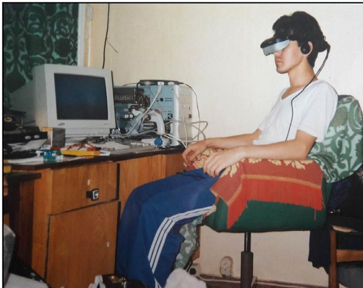
**1995, at the MAI campus, testing one of the world's first commercial VR harnesses, which ran at 640x480 @ 30fps. It used a magnetic sensor at the nape for head positioning. The best prank to play on someone was to bring a magnet near the rear side and shake it. It guaranteed screams when the 3D world rolled around!**
