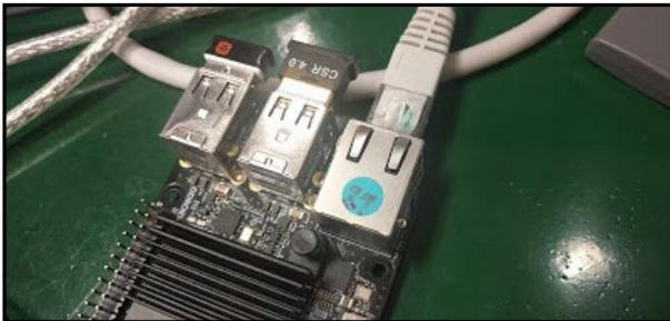
**ODROID with Bluetooth dongle on USB port**
