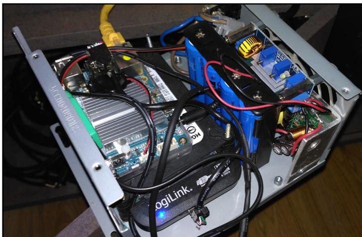
**Joachim's home server powered by an ODROID-C1, all tightly fitted into an old ATX power supply case**
